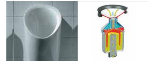
▲ Waterless Urinal uses the Erlenmeyer flask principle. The Urine itself helps to keep gases sealed in and prevent their escape
